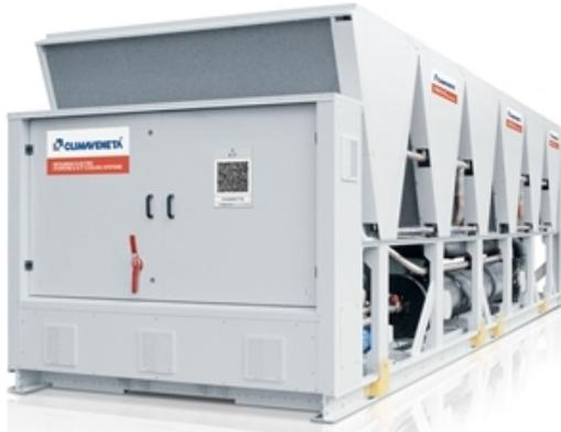
Outdoor unit for the production of chilled water with semi-hermetic screw compressor optimized for R513A, axial-flow fans, micro-channel full-aluminum condensing coils, single-pass shell and tubes evaporator designed by Mitsubishi Electric Hydronics & IT Cooling Systems S.p.A. (brazed plate evaporator for sizes 0751 and 0851) and electronic expansion valve. Base and supporting structure and panels are of galvanized epoxy powder coated steel with increased thickness. Eurovent certification.
