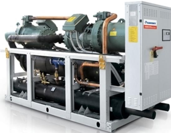
**Unit for indoor installation for chilled water production. Semihermetic screw compressors optimized to operate with low compression ratio and R513A; shell and tubes condenser and direct expansion evaporator; electronic expansion valve. Frame in polyester-painted galvanized steel. High efficiency unit: the innovative optimized compressors and the high performing heat exchangers enhance EER values up to 5,1 (CA version) and even up to 5,6 (CA-E version) at Eurovent standards conditions.**
