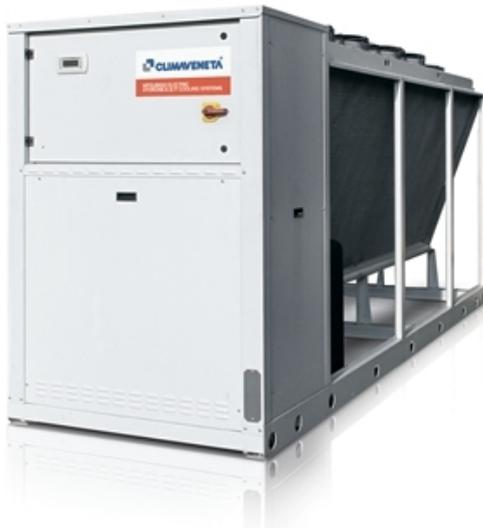
**Outdoor unit for the production of chilled water with hermetic rotary Scroll compressors, ozone-friendly refrigerant R410A, axial-flow fans, plate heat exchanger, micro-channel full-aluminum air coils and thermostatic or electronic expansion valve, according to the model. The range is composed by units equipped with two compressors in a single-circuit configuration.**
