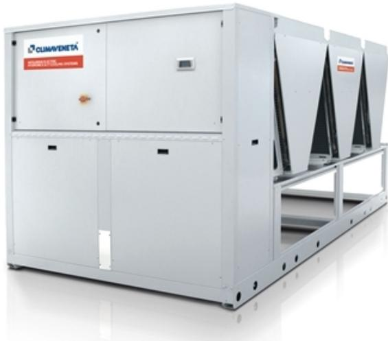
**Outdoor unit for the production of chilled water with hermetic rotary Scroll compressors, ozone-friendly refrigerant R410A, axial-flow fans, shell and tubes heat exchanger, micro-channel full-aluminum air coils and thermostatic or electronic expansion valve, according to the model. The range is composed by units equipped with four compressors in tandem configuration on two independent refrigeration circuits.**
