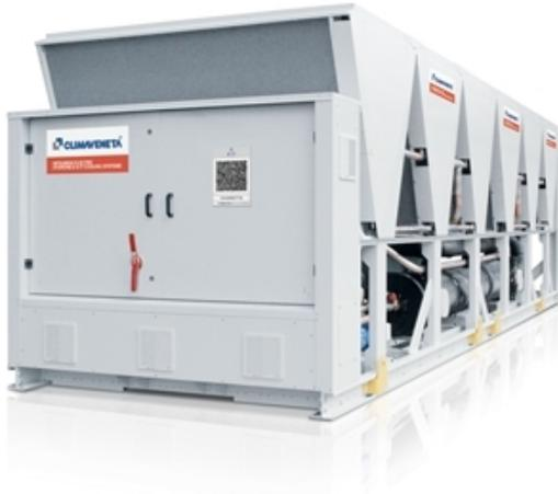
Outdoor unit for the production of chilled water with semi-hermetic screw compressors optimized for R134a, axial-flow fans, micro-channel full-aluminum condensing coils, single-pass shell and tubes evaporator designed by Mitsubishi Electric Hydronics & IT Cooling Systems S.p.A. and electronic expansion valve.
