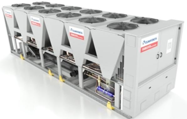
Outdoor unit for the production of chilled water with semi-hermetic variable-speed screw compressors optimized for HFO R1234ze refrigerant, axial-flow fans, micro-channel full-aluminum condensing coils, single-pass shell and tubes evaporator designed by Mitsubishi Electric Hydronics & IT Cooling Systems S.p.A. and electronic expansion valve.
