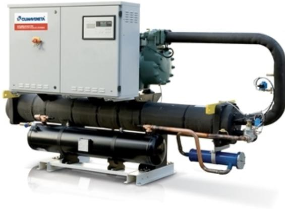
Indoor unit for the production of chilled water combined with a remote condenser, with semi-hermetic screw compressors optimized for R134a, shell and tube evaporator designed by Mitsubishi Electric Hydraulics & IT Cooling Systems S.p.A. and thermostatic expansion valve.
