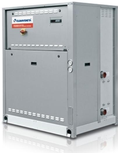
**Indoor unit for the production of chilled water that may be connected to a remote condenser with hermetic rotary scroll compressors working with R410A, braze-welded plate-type exchanger and thermal expansion valve. Panels and base in hot-dip galvanised sheet steel with paint finish.**
